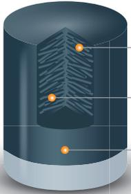
Copper oxide rods held together in wax matrix
